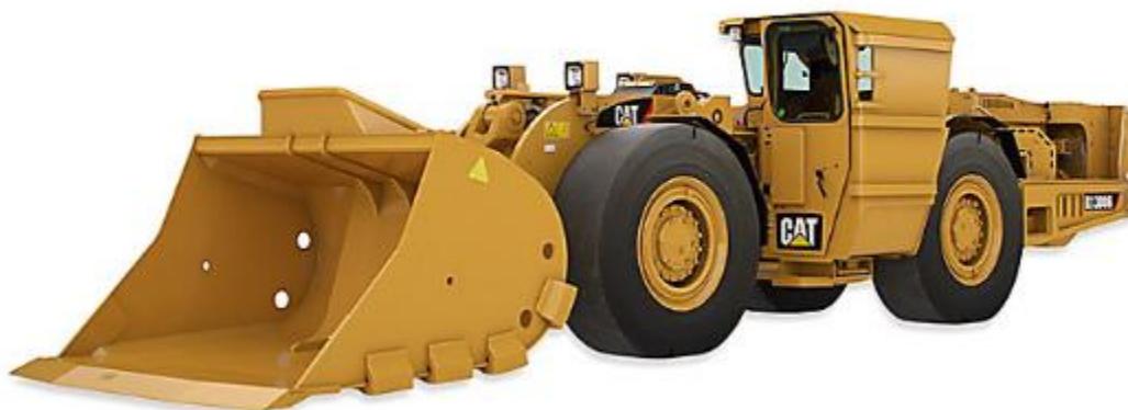
Figura 16. Scoop CAT R1300G Tomada de Caterpillar Performance Handbook. (12)
