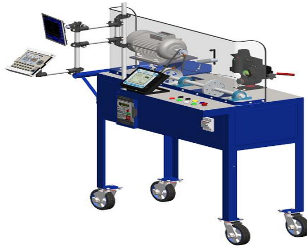
Figure 1. Prototype of the 3D design of the vibratory and thermographic test bench designed in Solidworks software.
